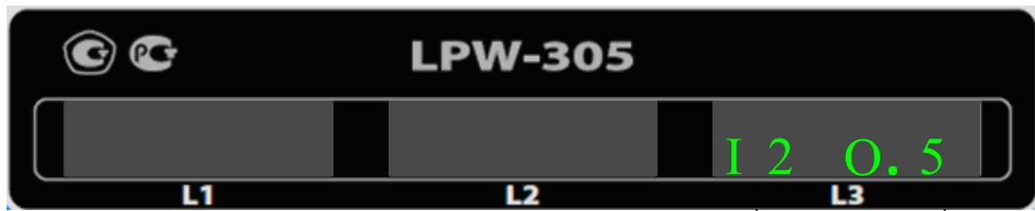
The overvoltage threshold is a number in the range from 101.0 to 150.0, per cent; change is made in increments of 0.1
