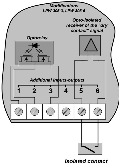
Figure B.16 – Connection of the mechanical contact to the discrete input of DIN-rail mounted LPW-305
