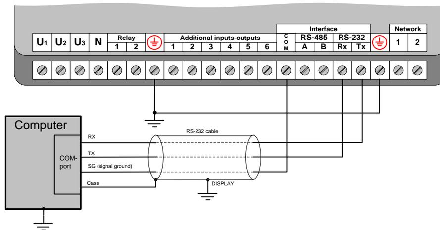
Figure B.11 – Connection of LPW-305 for DIN-rail mounted LPW-305 to the RS-232 interface
