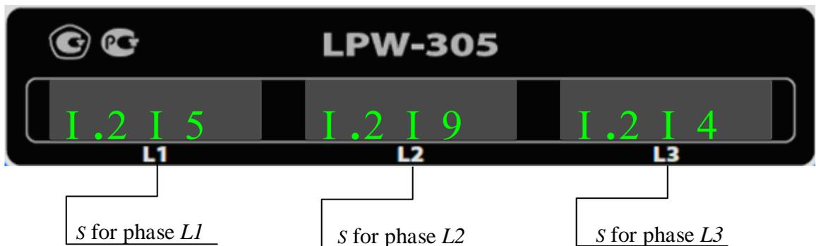
The dimension of the indicated value  $S$  can be changed by pressing the "SELECT" key.
