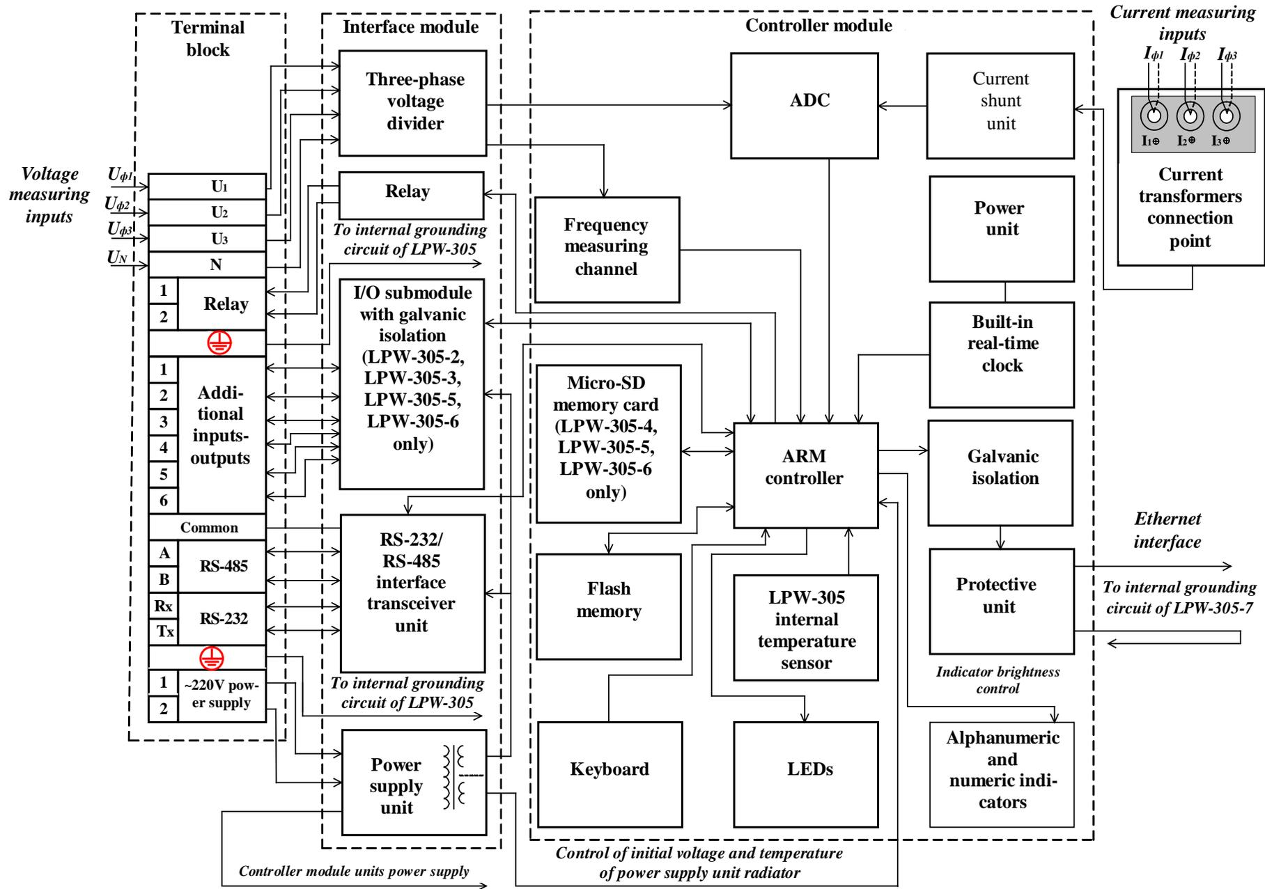
Figure 2 – Electrical block diagram of DIN-rail mounted LPW-305
