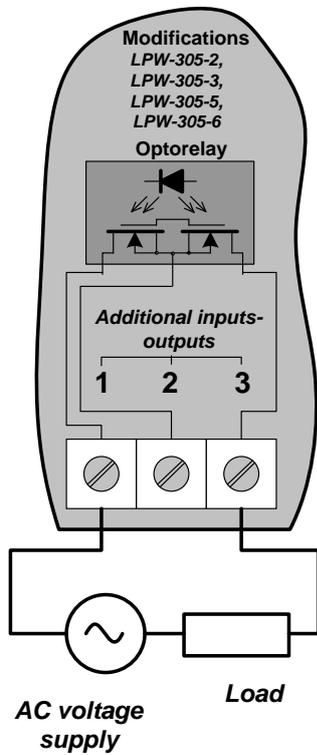
Figure B.13 – Connection of the pulse output of opto-relay of DIN-rail mounted LPW-305 to an AC circuit
