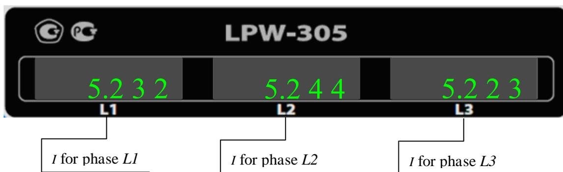
The dimension of the indicated value  $I$  can be changed by pressing the "SELECT" key.
