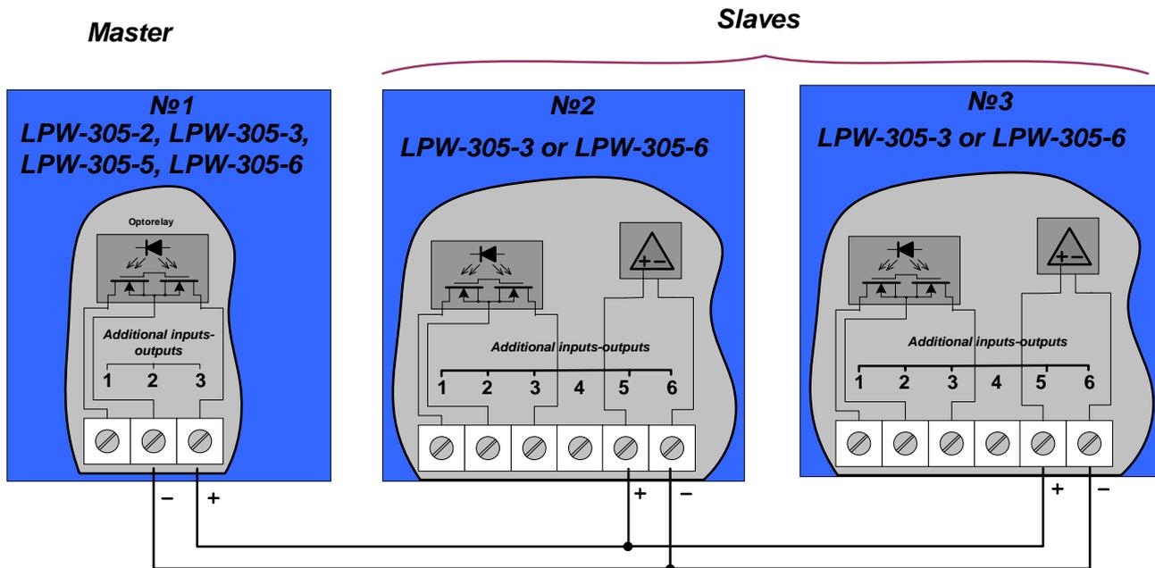
Figure B.18 – Signaling based on the "master-slave" principle- for DIN-rail mounted LPW-305
