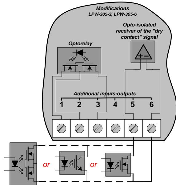
Figure B.17 – Options for connection of "electronic contacts" to the discrete input of DIN-rail mounted LPW-305
