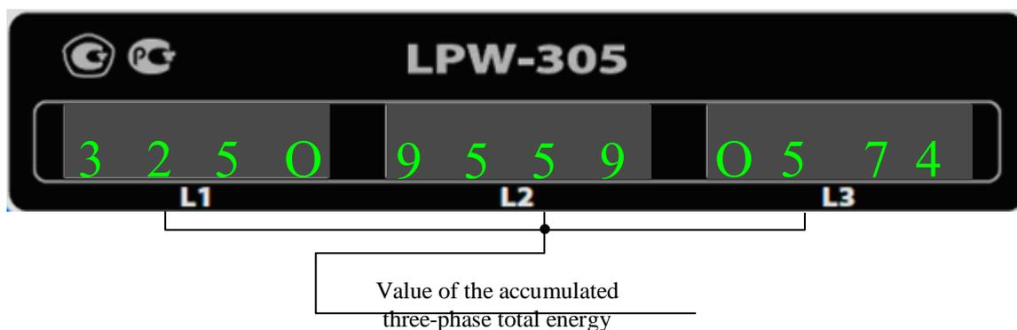
For displaying, the three indicators are combined into one, thus forming a single indicator for 12 positions.
