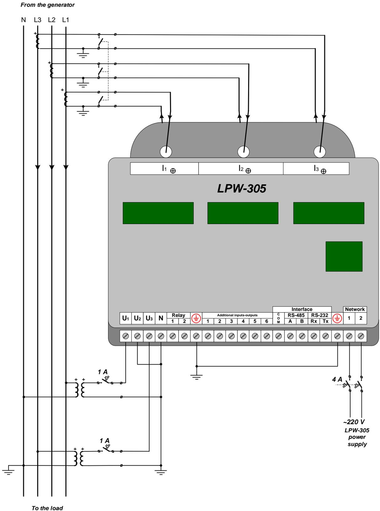
Figure B.3 – Diagram of four-wire "star" connection with three CTs and two VTs, for DIN-rail mounted LPW-305
