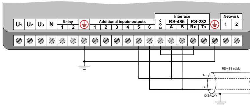
Figure B.10 – Connection of LPW-305-2 and LPW-305-5 modifications to the RS-485 interface line as a device with 120 Ohm line load
