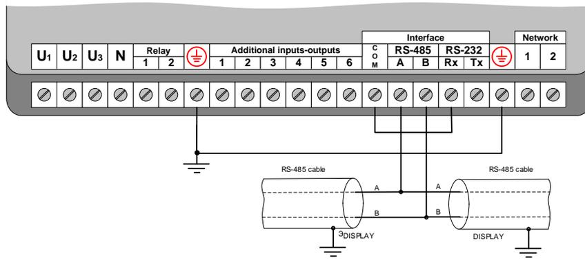
Figure B.8 – Connection of DIN-rail mounted LPW-305 to RS-485 interface as a transmission device
