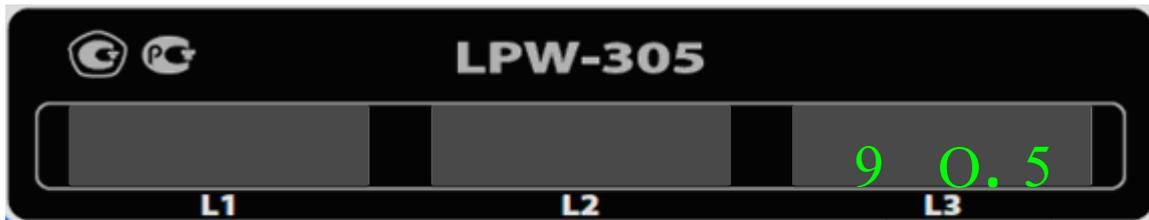
Voltage fall threshold is a number in the range from 10.0 to 99.0, per cent, change is made in increments of 0.1
