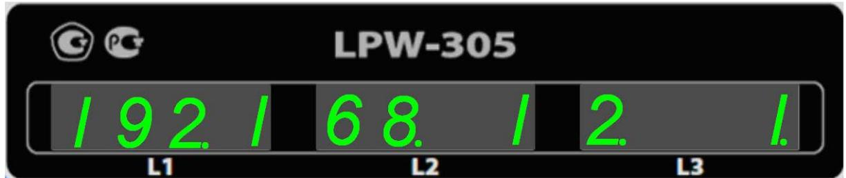
Gateway address consists of four groups of digits. Each group is an integer from 0 to 255 with a point at the end.
