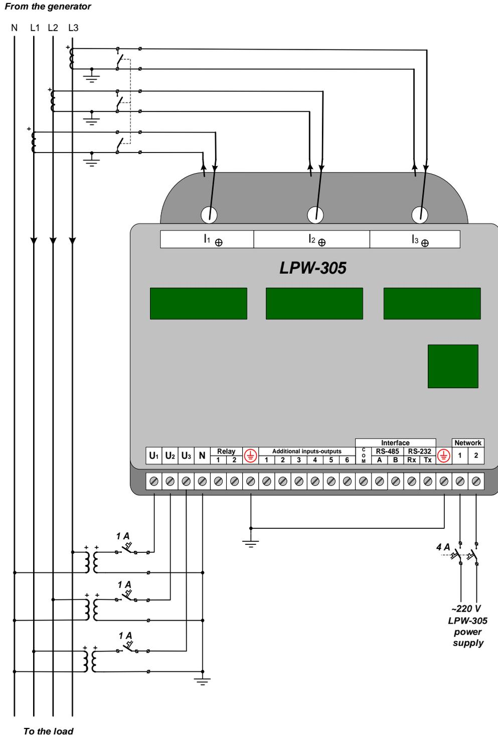
Figure B.1 – Diagram of four-wire "star" connection with three CTs and three VTs, for
