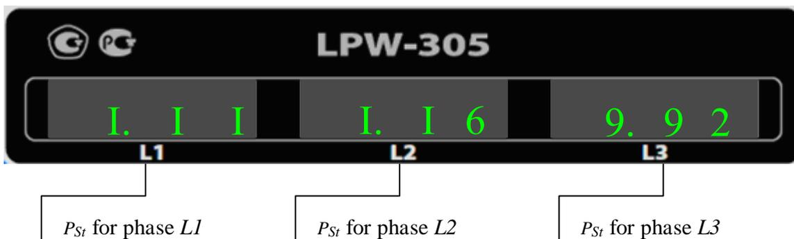
If the indicated value of short-term flicker indicator value  $P_{St}$  falls out the measurement range indicated in paragraph 2.5, then the indicator state is the following:
