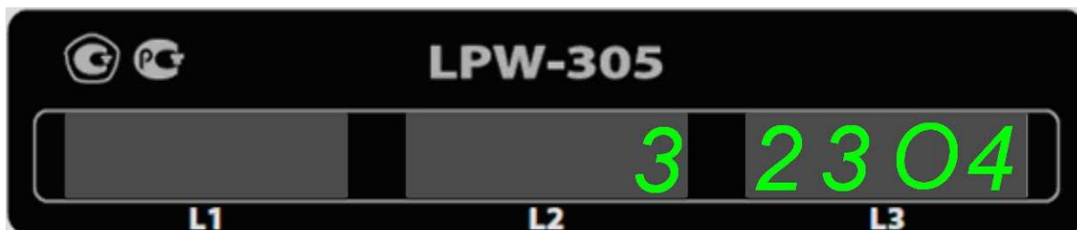
The correction factor for current measurement results is an integer in the range from 1 to 50000; change is made in increments of 0.1
