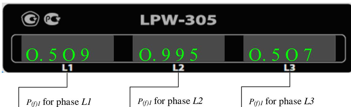
The dimension of the indicated value  $P_{(f)1}$  can be changed by pressing the "SELECT" key.
