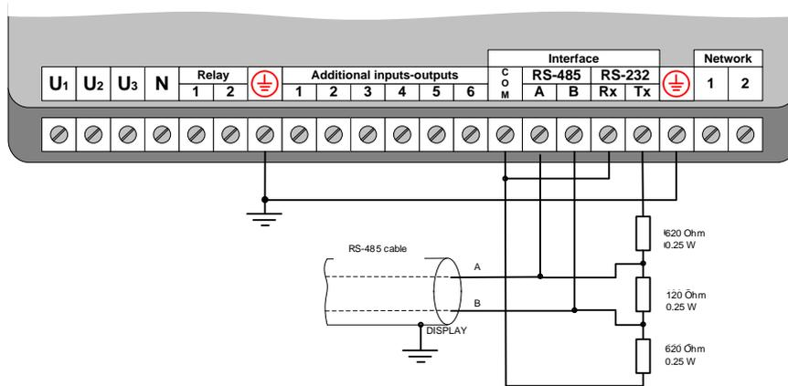
Figure B.9 – Connection of DIN-rail mounted LPW-305 to RS-485 interface as a termination device
