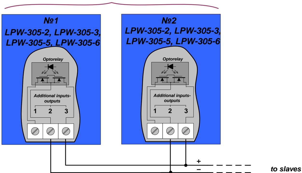
Figure B.19 – Connection of master LPW-305 mounted on DIN-rail in a signaling circuit based on the "logic OR" principle
