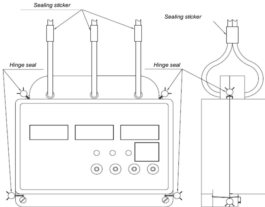
Figure 3 – Sealing of DIN-rail mounted LPW-305
