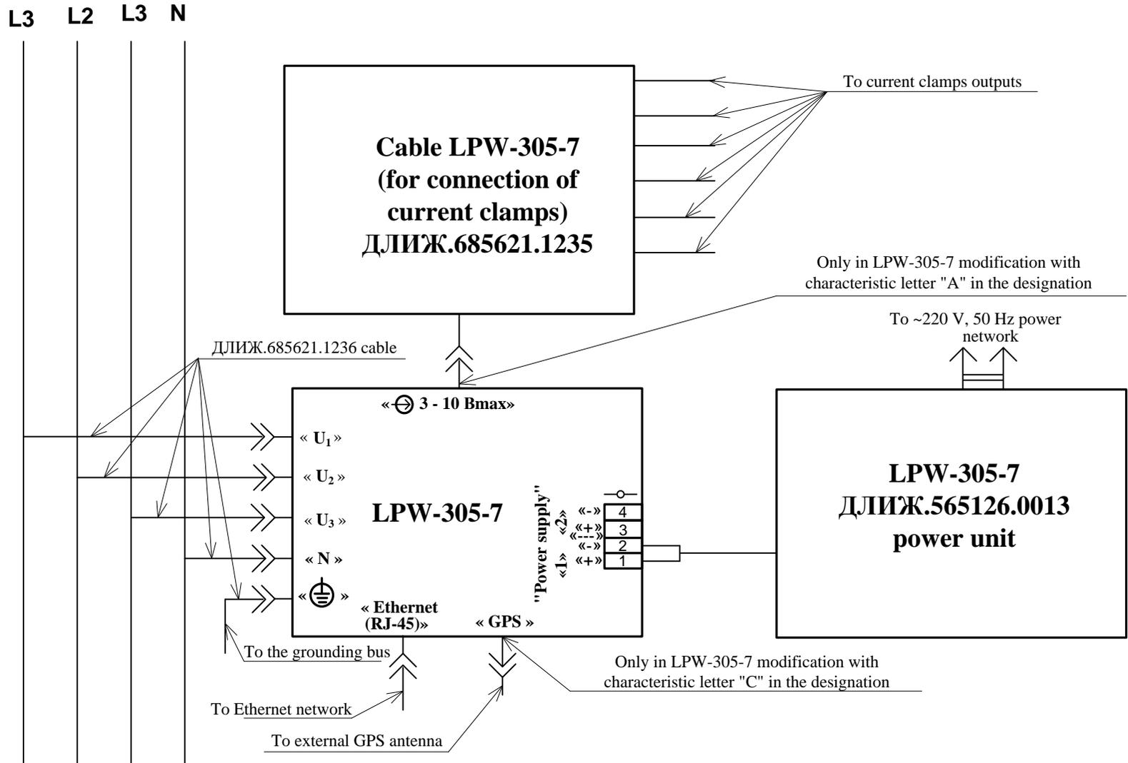
Figure B.21- Electrical block diagram of four-wire LPW-305-7 connection
