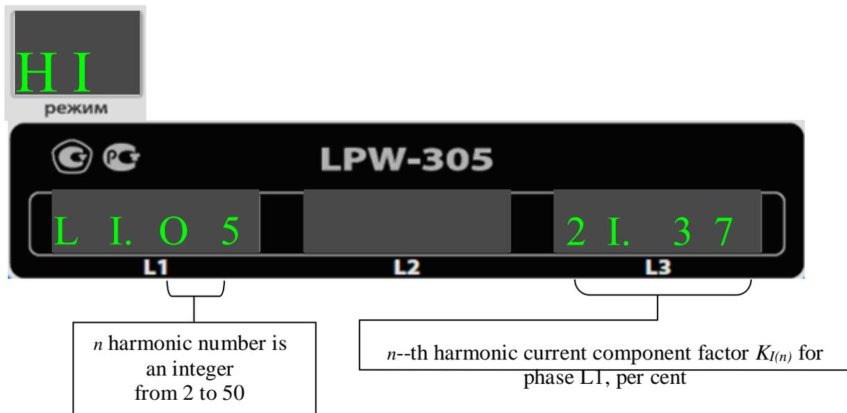
The third and fourth positions of the leftmost indicator are used to display the harmonic number, the harmonic component for which is displayed on the rightmost indicator.
