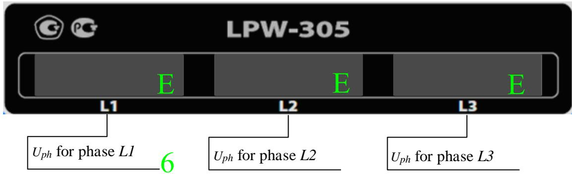
7.3.4 Indication of the value of the phase shift angle  $\varphi_U$  between the phase voltages of the fundamental frequency (first harmonic) relative to phase L1 (item "00." of the main menu, the item " $\angle U$ " of the sub-menu)
