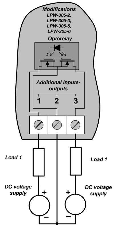
Figure B.15 – Connection of the pulse output of opto-relay of DIN-rail mounted LPW-305 to two DC circuits
