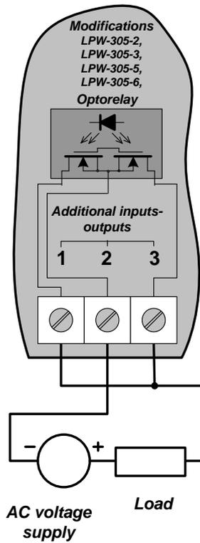
Figure B.14 – Connection of the pulse output of opto-relay of DIN-rail mounted LPW-305 to a DC circuit
