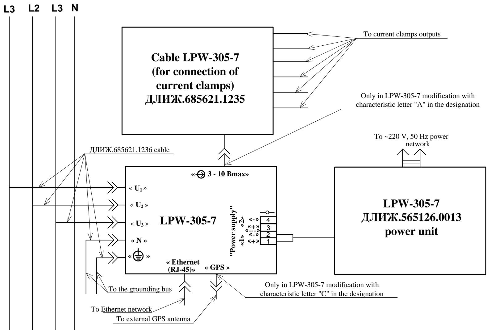
Figure B.22- Electrical block diagram of four-wire LPW-305-7 connection
