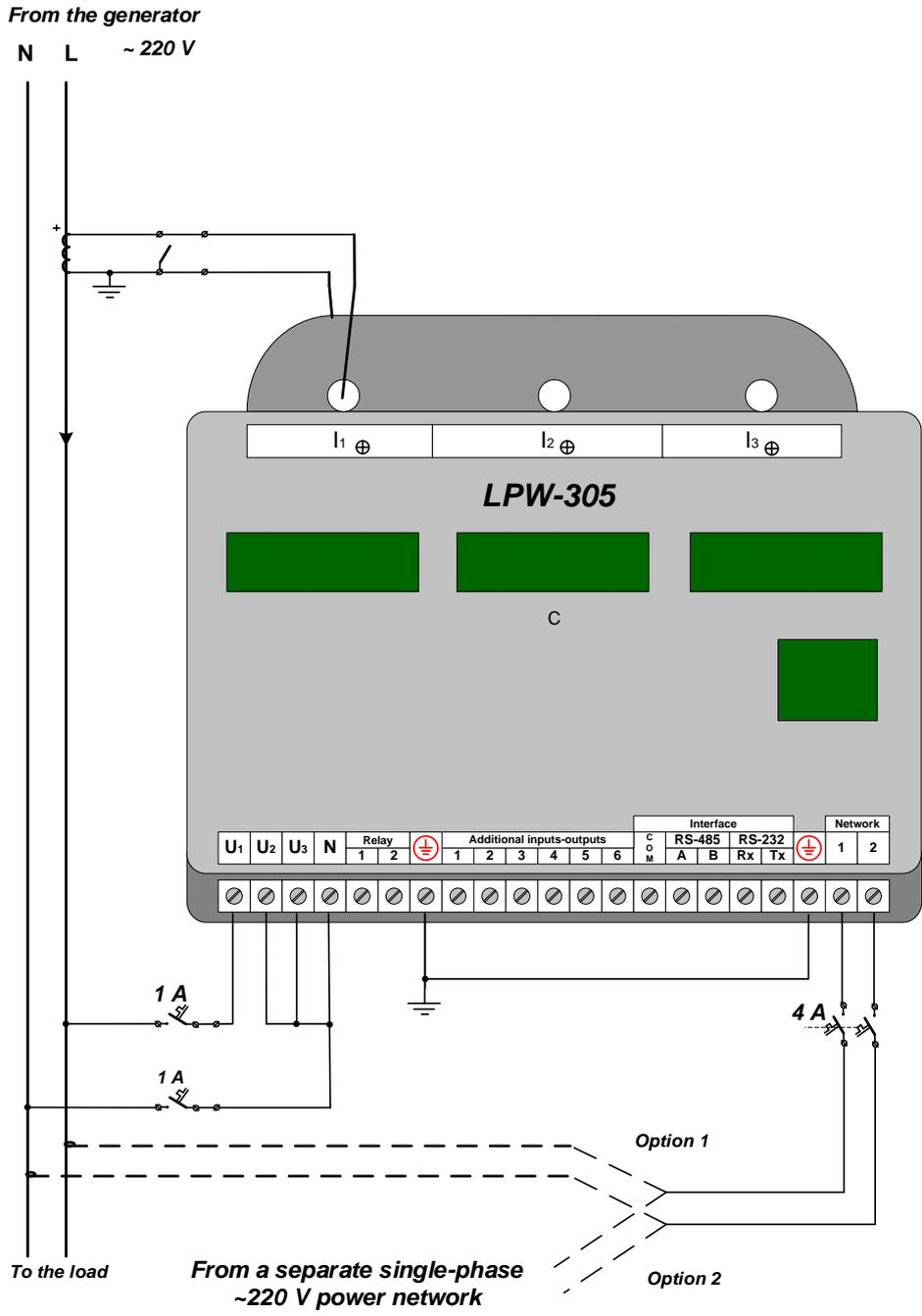
Figure B.7 – Diagram of connection to a single-phase network with two power supply options: either from a separate network or from a measuring circuit, for DIN-rail mounted LPW-305
