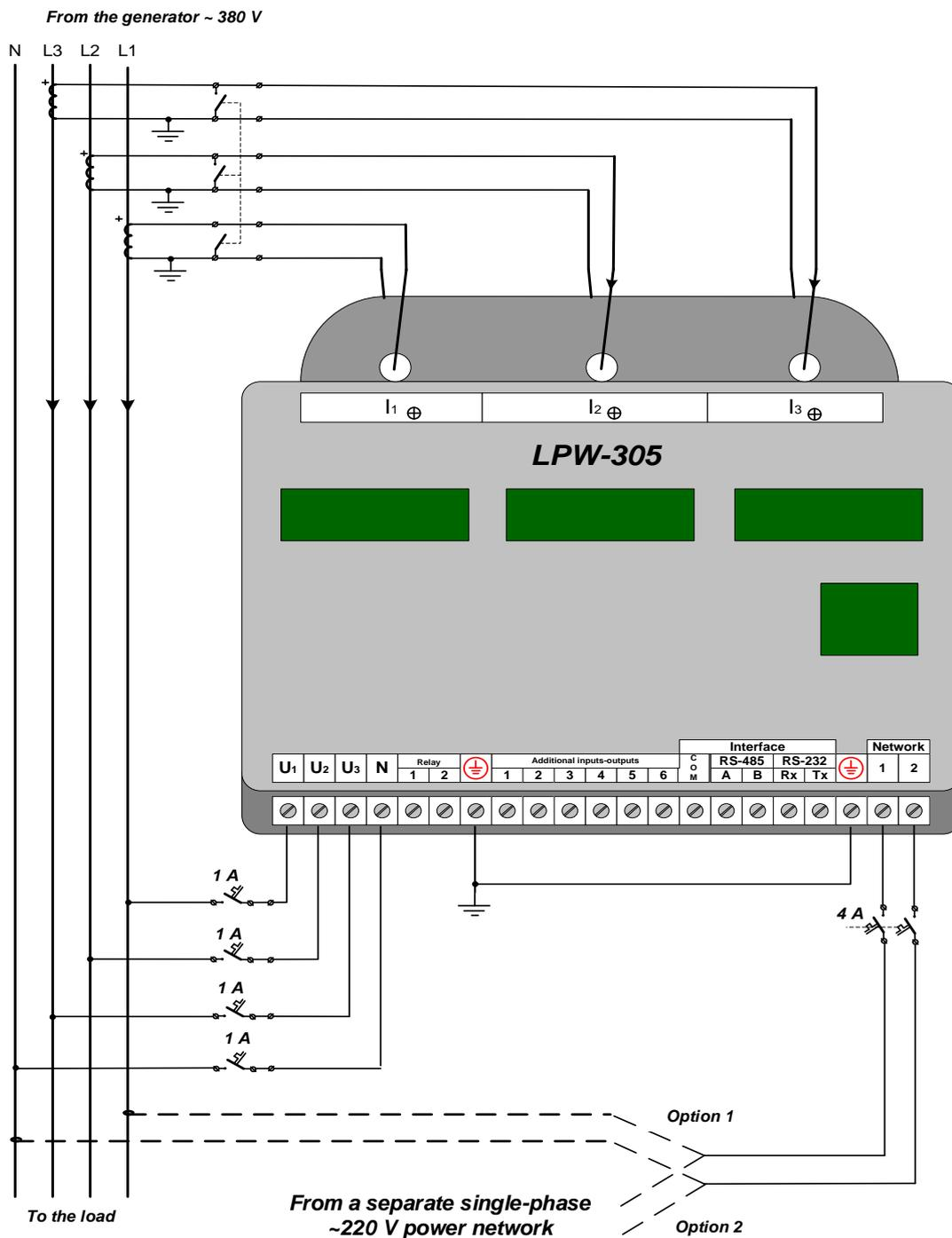
Figure B.2 – Diagram of four-wire connection with three CTs and two power supply options: either from a separate network or from one of voltage measuring circuit phases for DIN-rail mounted LPW-305
