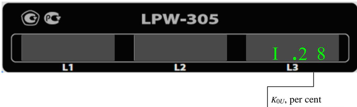
If the indicated value of zero sequence unbalance factor  $K_{0U}$  falls out the measurement range indicated in paragraph 2.5, then the indicator state is the following:
