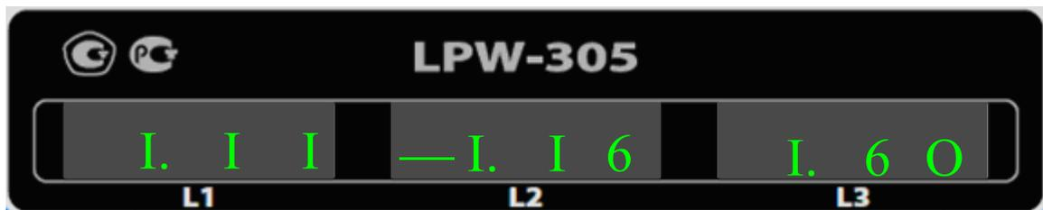
Aggregate (for three phases) active power value
