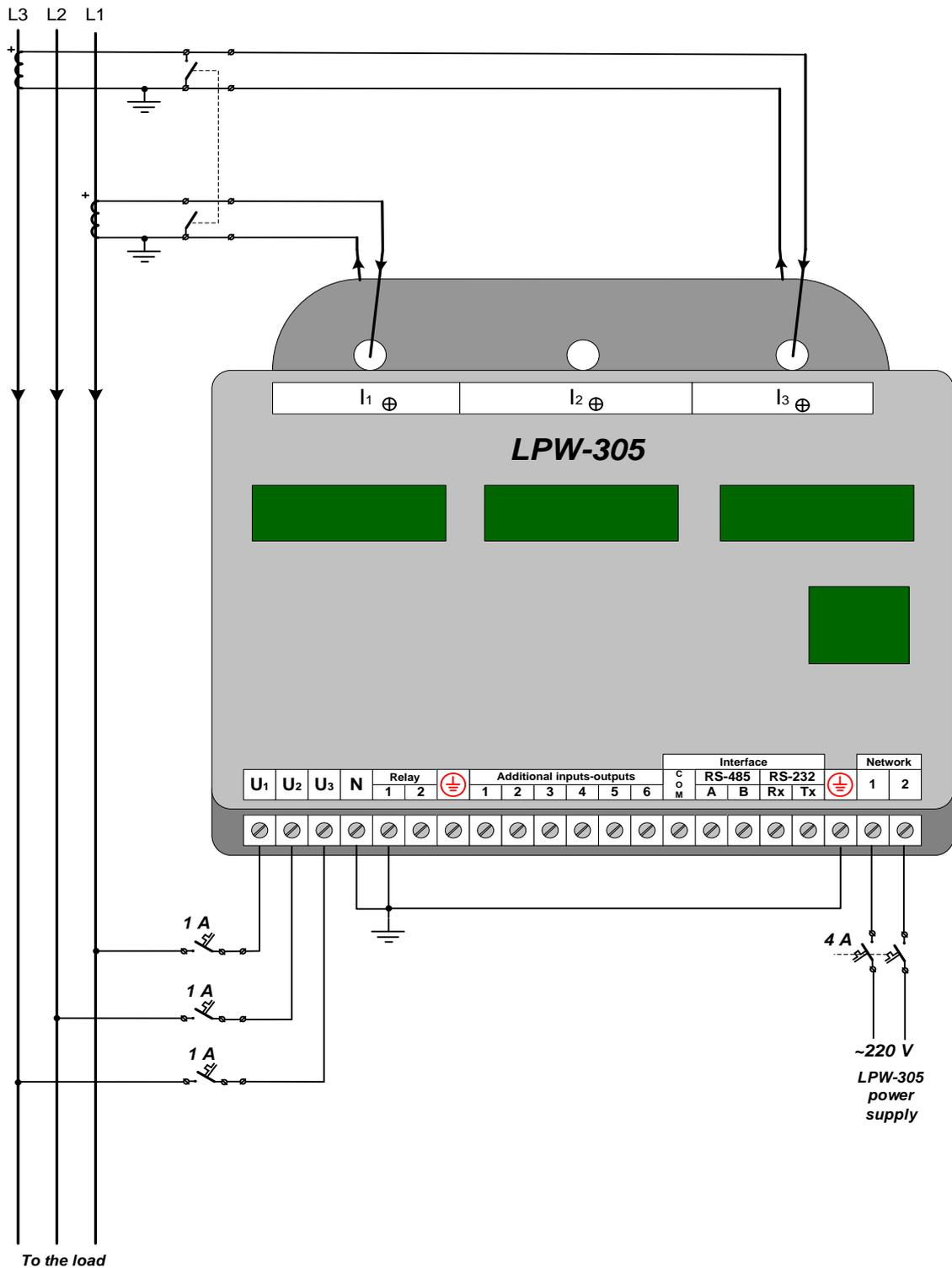
Figure B.4 – Diagram of three-wire connection with two CTs,
