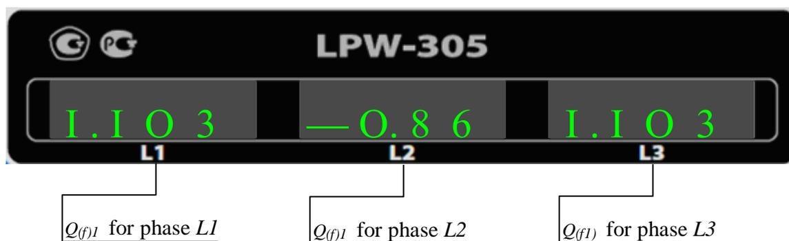
The dimension of the indicated value  $Q_{(f)1}$  can be changed by pressing the "SELECT" key.
