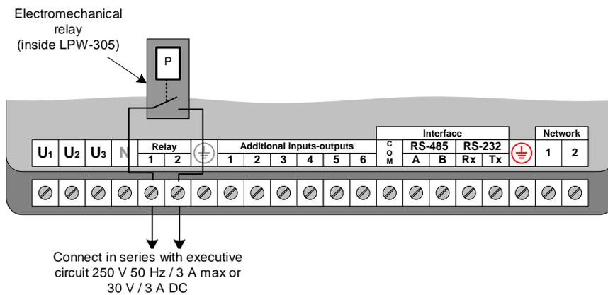
Figure B.12 – Connection to the contacts of electromechanical relay for DIN-rail mounted LPW-305
